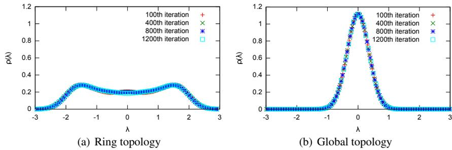
**Fig. 5** Density spectrum of the swarm influence graph for the static topologies.
